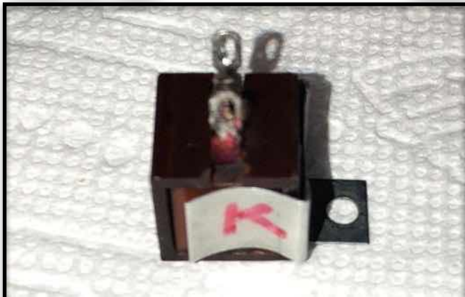
Figure 7: Completed Selenium Rectifier Converted to Silicon with Cathode Marked
