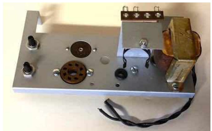
Figure 6: The V-6 chassis, cleaned, coated and partially populated with parts.
