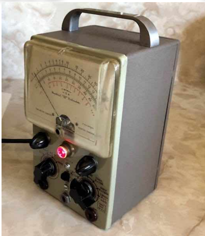
Figure 2: Another photo of the completed restoration of the Heathkit V-6 VTVM during burn-in. This photo shows the repainted case color.
