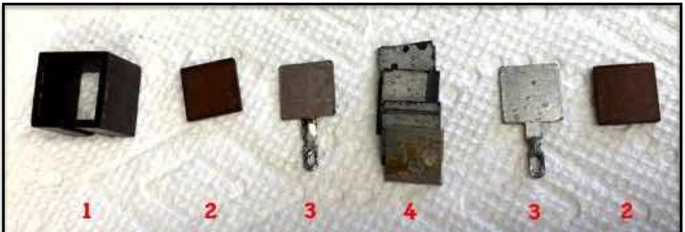
Figure 3: The disassembled 57-1 Rectifier.
