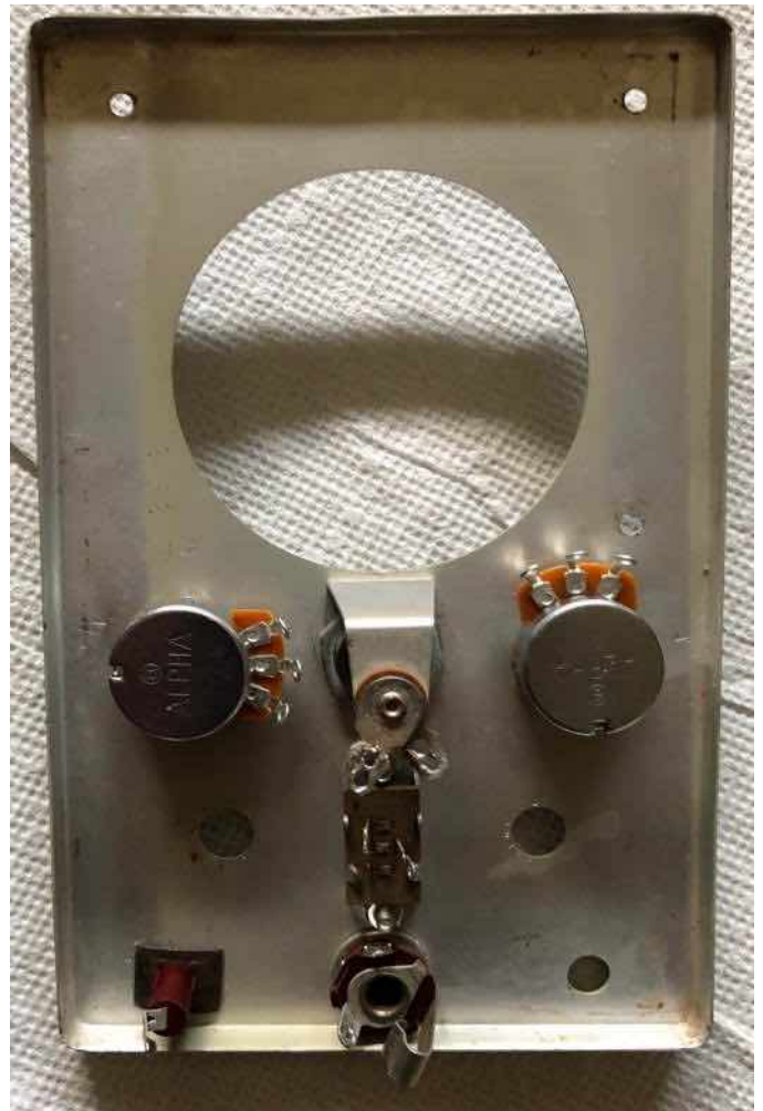
Figure 8: The front panel rear with ZERO ADJ. and OHMS ADJ. controls, pilot lamp, D.C. jack, A.C. - OHMS jack and OFF - ON switch installed.
