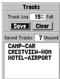
The Tracks Page with a list of saved tracks. Tracks that are not named are assigned a date.
