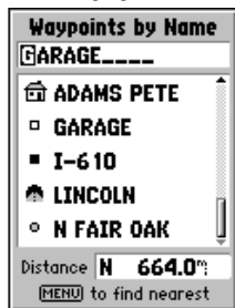
Waypoints By Name List. Use the ROCKER keypad to enter the first characters of the waypoint name or scroll through the list.
