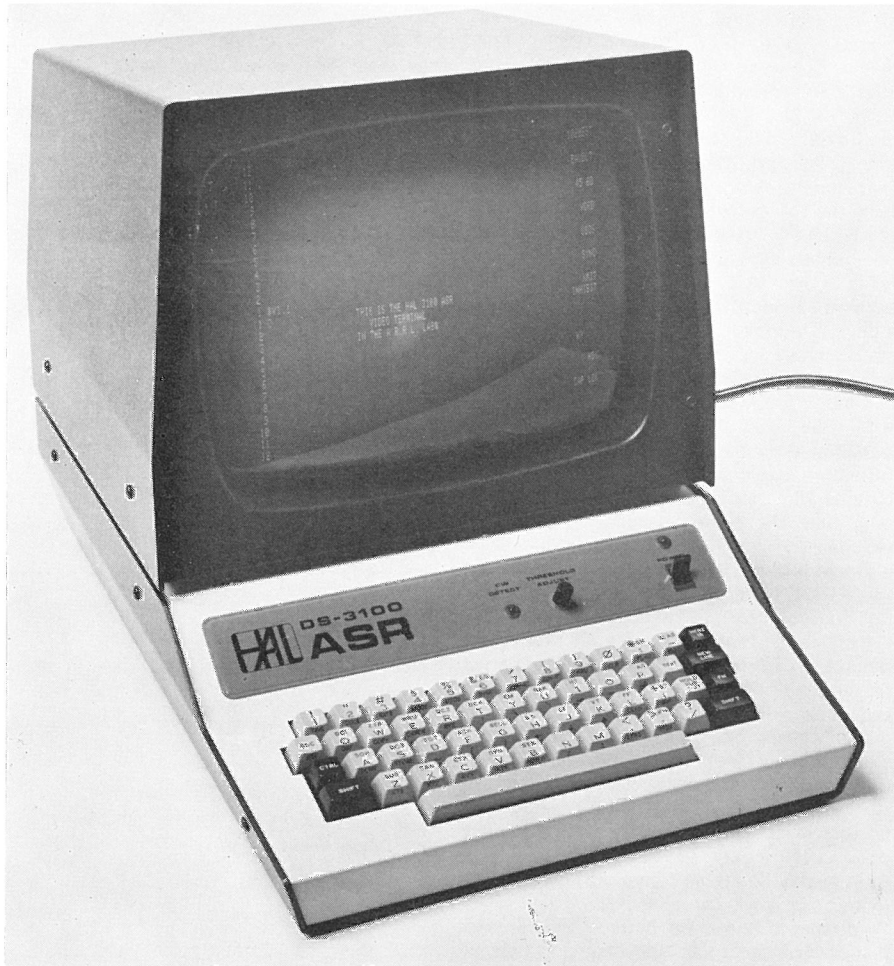
The HAL DS3100 ASR Video Display Terminal. This completely buffered terminal offers a multitude of features for completely automated transmission and reception of Morse, Baudot and ASCII RTTY.
