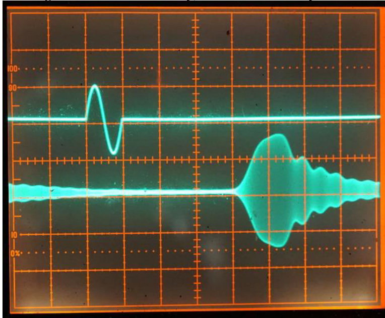
Figure 36: Transmit latency, MID TBW. Latency 4.2 ms.
