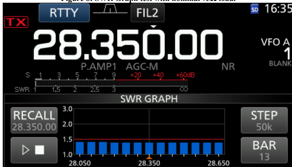
Figure 8: SWR Graph test with nominal 75Ω load.
