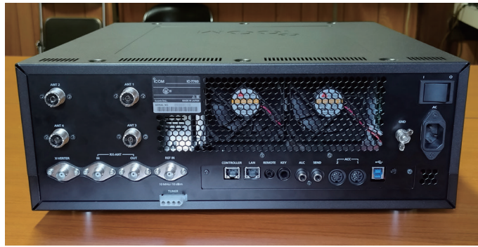
Figure 07-2. Rear panel of the RF deck
