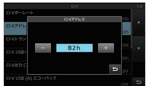
Figure 07-8. IC-7760 CI-V address
