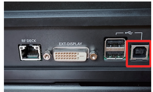
Figure 07-6. Connect a USB cable to the USB port on the controller's rear panel (red squared)
