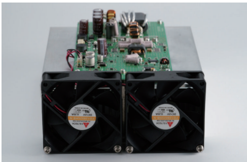
Figure 05-15. Two large cooling fans are installed on the PA unit
