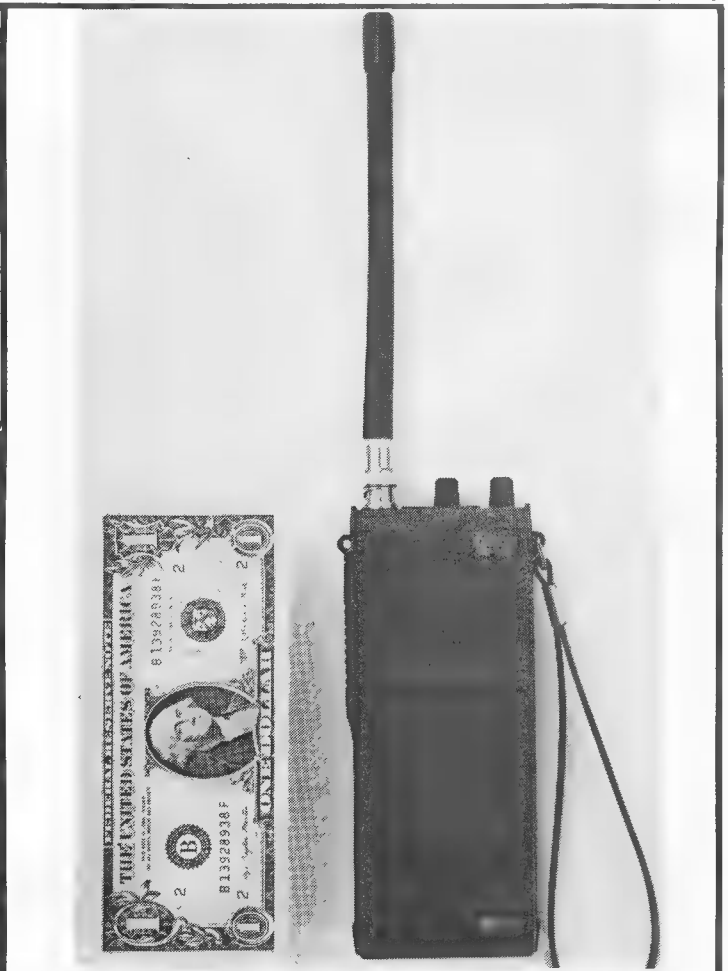
Although the IC-2A is small, the unit is crammed with components as PHOTO 3 (left) shows. The size of the unit is best described in PHOTO 4 (right) where the unit's size is compared to an American dollar bill.
