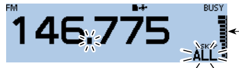
The S-meter displays the received signal strength.
