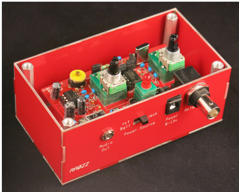
Figure 6.1 – Board Mounted in Enclosure
