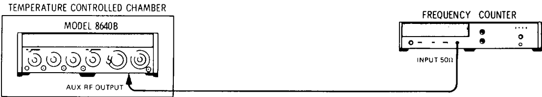
Figure 4-2. Frequency stability vs Temperature Test Setup
