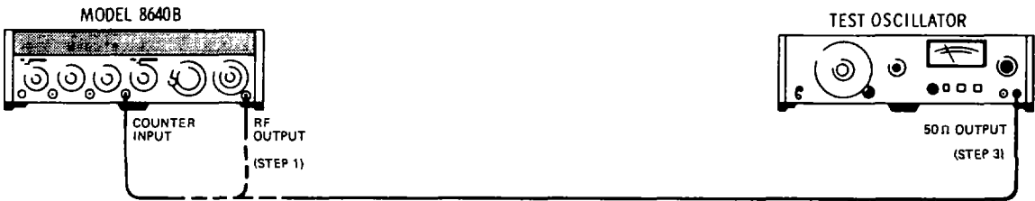
Figure 4-28. Counter External Sensitivity Test Setup
