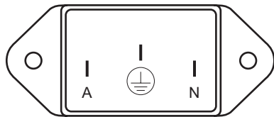
Figure 7: Front view of the IEC mains connector (10 A) on the power supply
