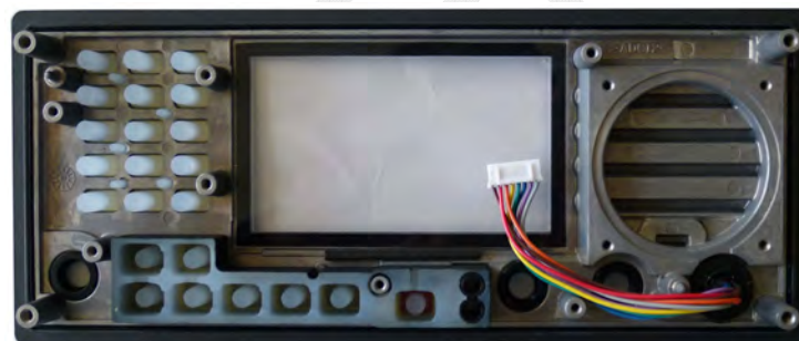
Fig. 2.1.7 Front panel, PANEL board removed
