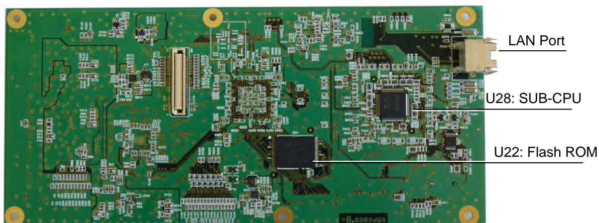
Fig. 2.5.42 T-CPU board (05P0859) B-side
