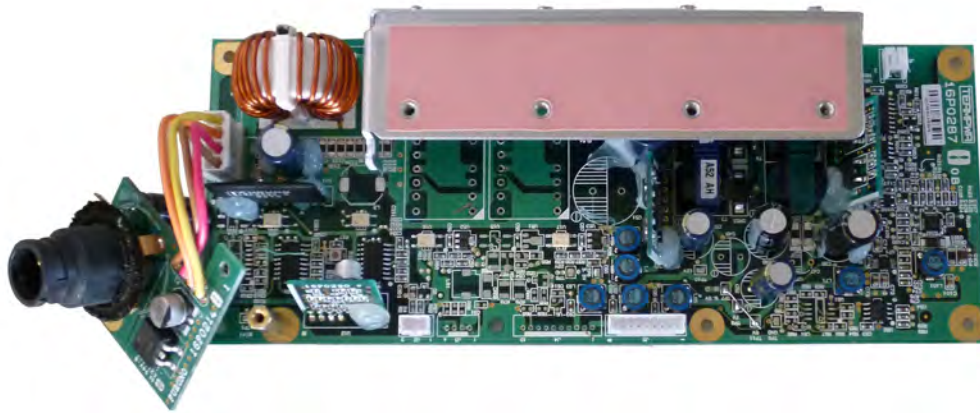
Fig. 2.7.18 TERM PWR board (16P0287A) A-side
