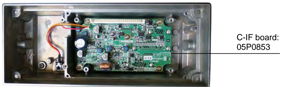
Fig. 2.1.5 Rear panel, C-CPU board removed
