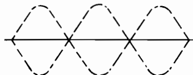
RF PATTERN SHOWING PROPERLY ADJUSTED PA BIAS
