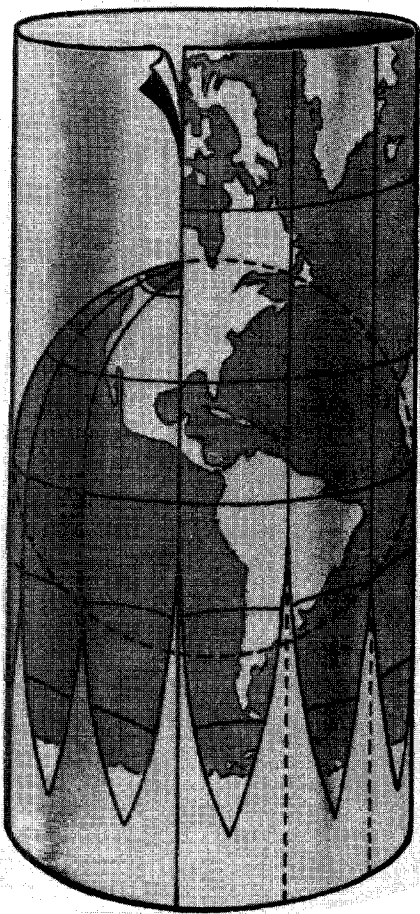
Figure 5-6. Mercator projection on a cylinder indicating method and showing polar distortion.
