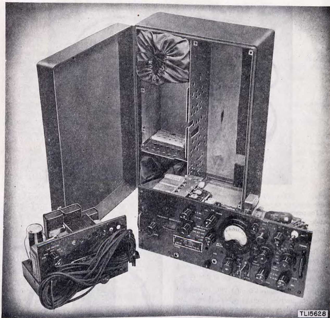
Figure 8. Rectifier Power Unit PP-36( )/PRC-1 and Receiver-Transmitter RT-30( )/PRC-1.
