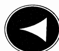
AM pattern excessive bias on 5894 stage.
