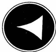
SSB pattern excessive bias on 5894 stage.
