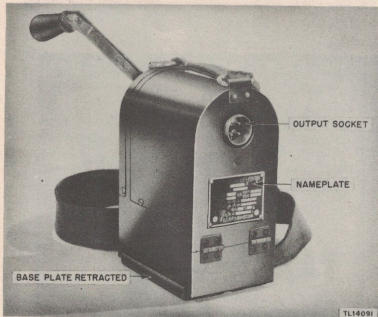
Figure 7. Model 97 Light Wireless Set manually operated generator, rear view.
