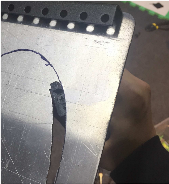
The speaker was secured by four flat head screws, whose heads were later painted black with a sharpie pen.
