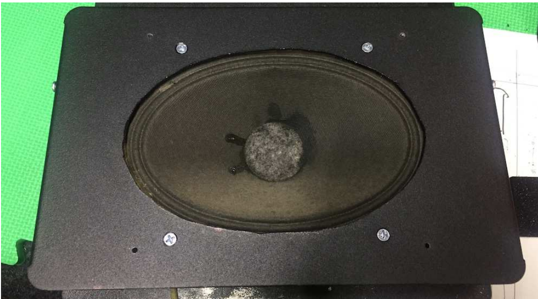
The grille plate was washed and dried on a stove before spray painted in several layers of black primer. A clear coat was sprayed after that. Four smaller screws hold the plate to the front panel.
