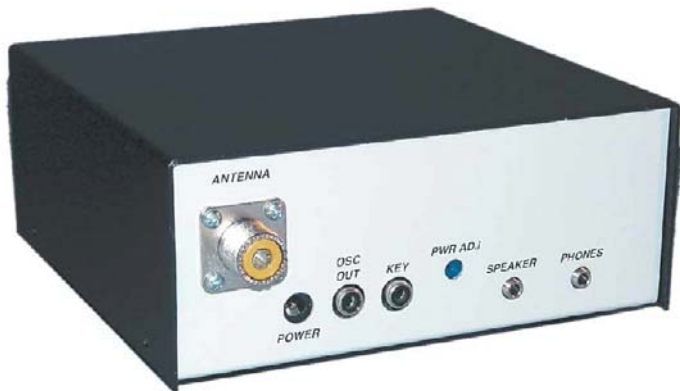
At the rear are jacks for (l-r) antenna, 12 V power, oscillator output (for frequency counter or digital dial), key line, power adjustment, speaker and headphones.
