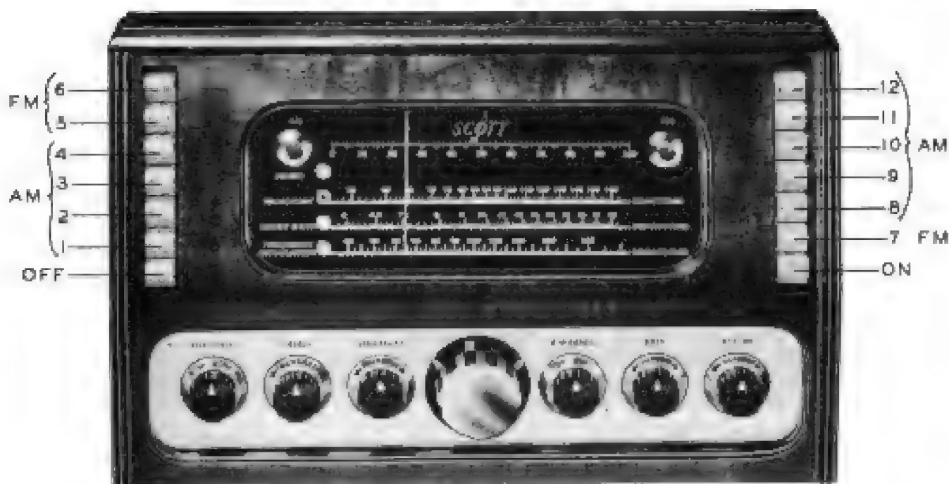
Figure 9 Front View 800-B Receiver Showing Pushbutton Sequence
