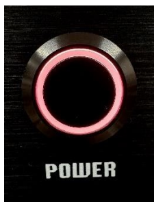
Power switch with Raspberry Pi running
