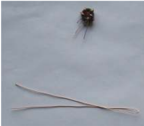
Figure 12: 20 cm of wire bent in half and shown beside a completed transformer
