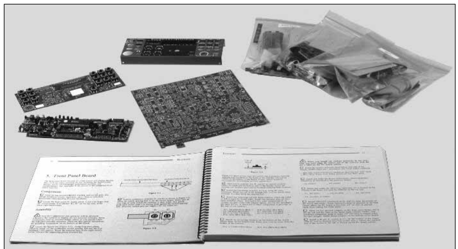
Figure 4—The three main circuit boards and their corresponding parts bags. At this stage I had completed the control board and was working on the display board.
