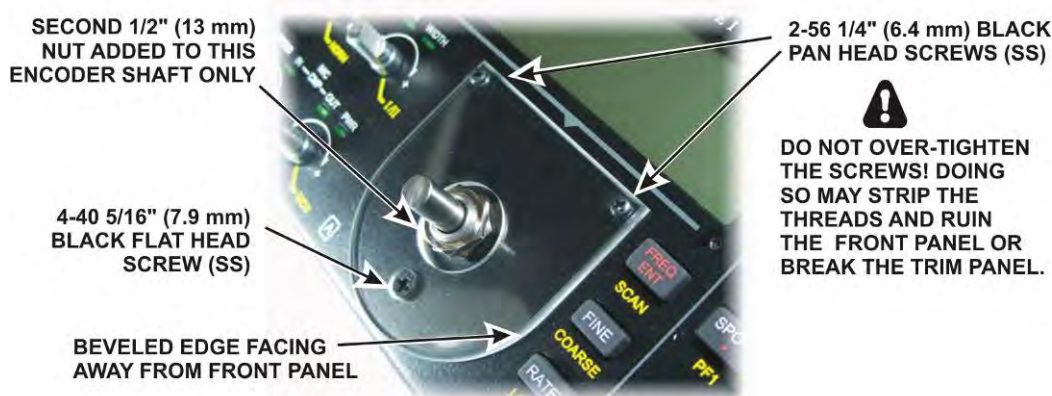
Figure 45. Mounting VFO A Trim Panel.
