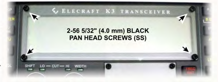
Figure 47. Installing LCD Cover.
