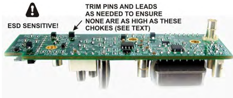
Figure 70. Checking Lead Lengths on KREF3 Board.
