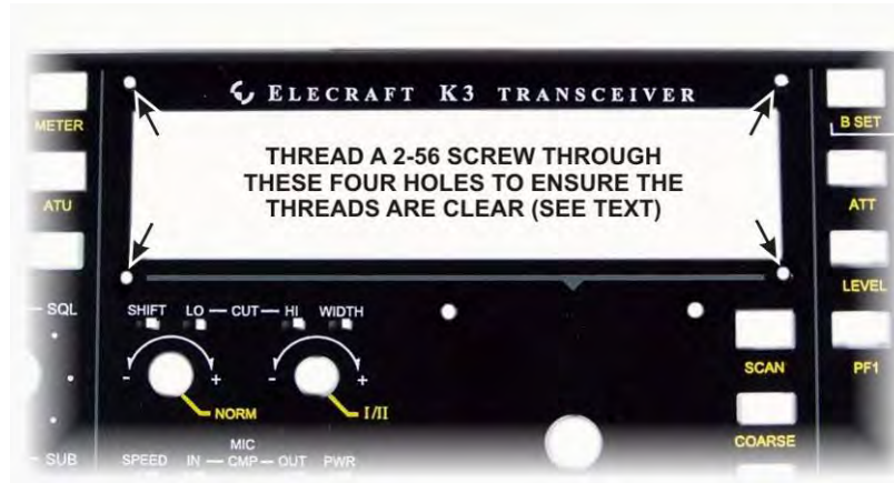
Figure 40. Checking 2-56 Threaded Screw Holes.
