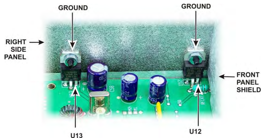
Figure 67. U12 and U13 Test Points.
