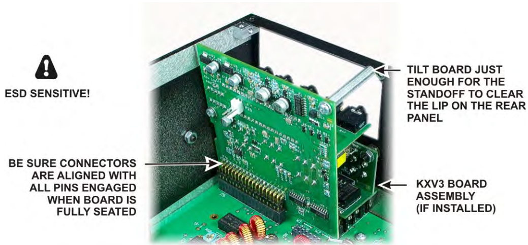
Figure 34. Installing KIO3 Main Board.
