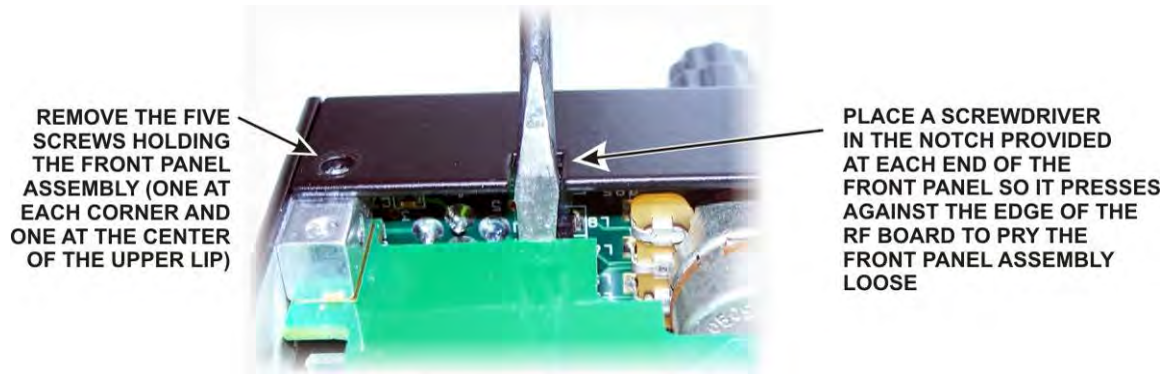
Figure 64. Removing the Front Panel.
