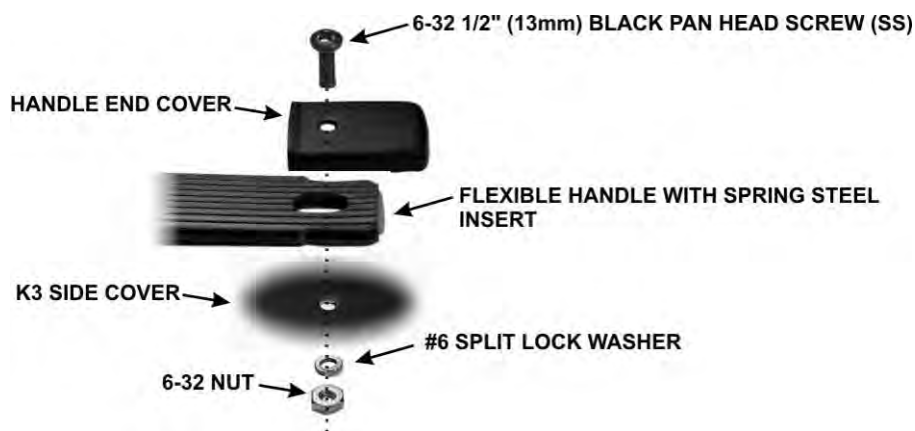
Figure 15. Installing Side Handle Mounting Hardware.
