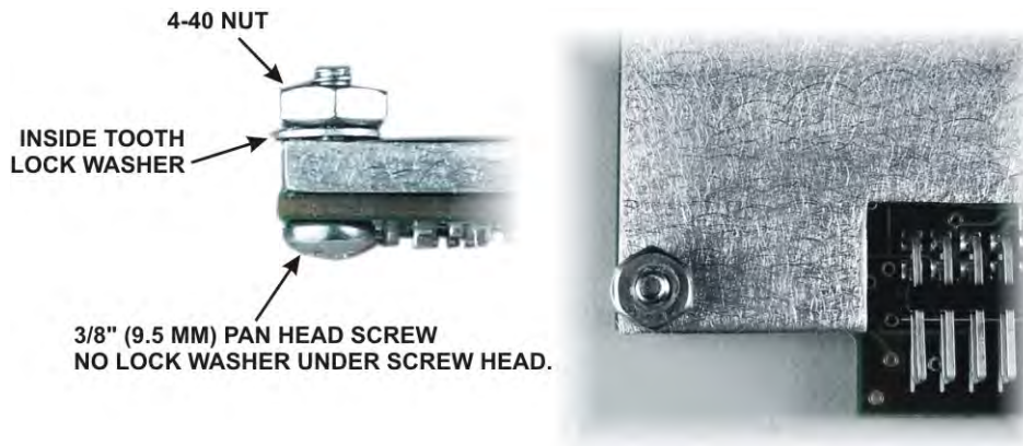
Figure 72 Stiffener Fastener on KSYN3 Board.
