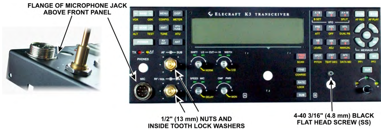
Figure 41. Mounting the Front Panel on the Front Panel Board.
