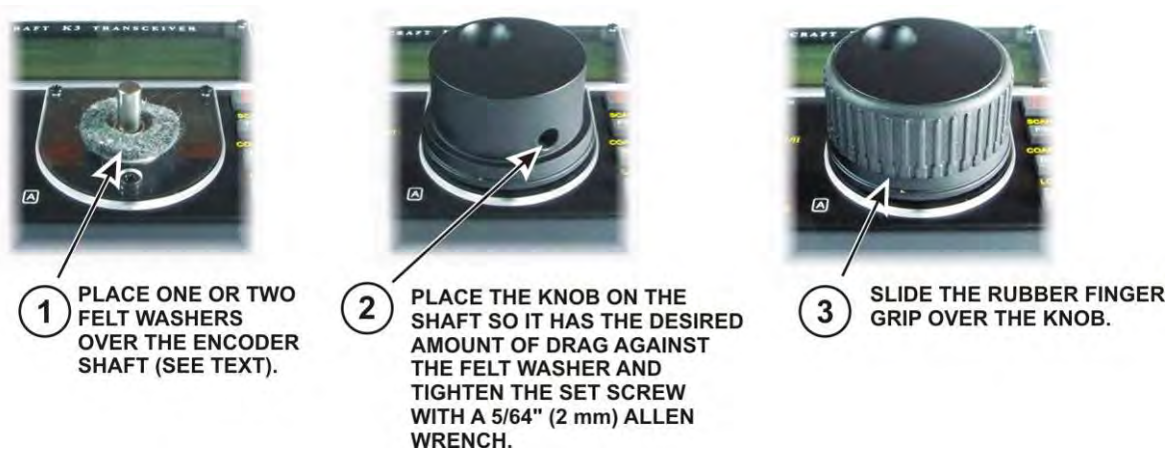
Figure 50. Mounting the VFO A Tuning Knob.
