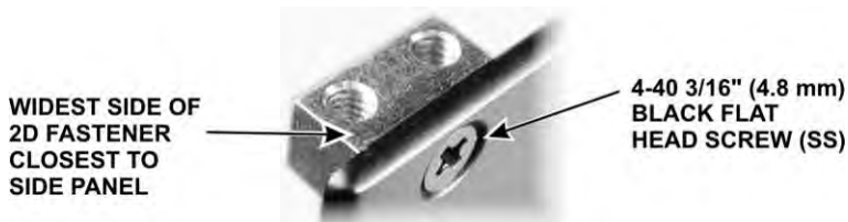
Figure 17. Installing Left Side Panel 2D Fastener.
