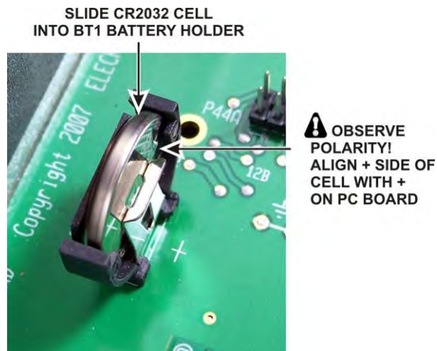
Figure 88. Installing BT1.
