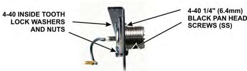
Figure 18. Mounting the ANT1 Connector.
