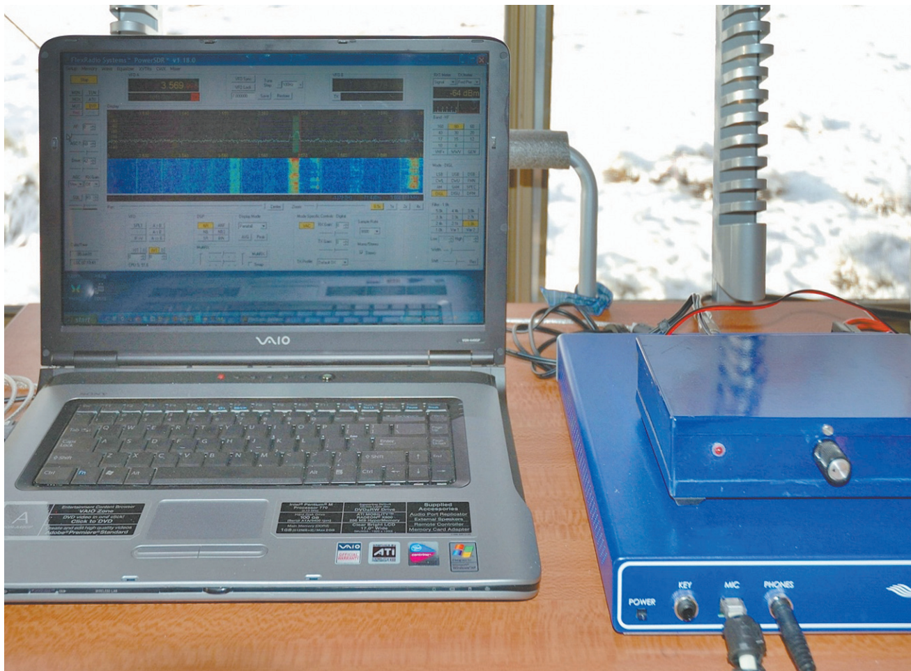
Photo 3: A photo of the complete station, with the 10 + 10 watt external audio amplifier (referred to in the text) sitting on top of the Flex-3000.
