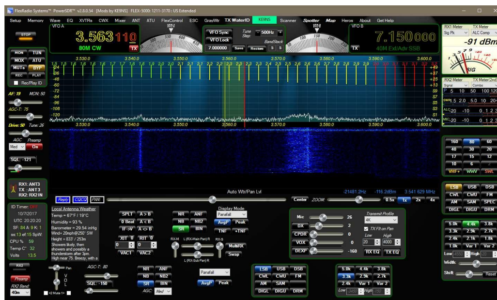
Showing the SWR scan results when "Display Recording SWR Plot(s) to Pan" is checked
