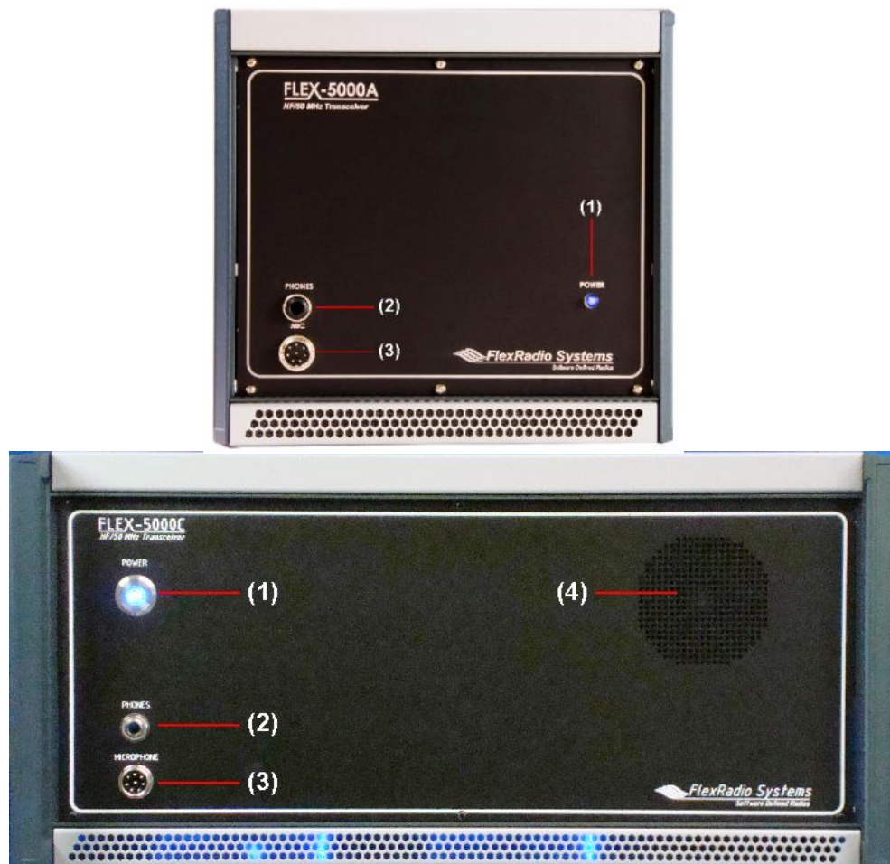
Figure 2: FLEX-5000A (top) and FLEX-5000C (bottom) Front Panel
