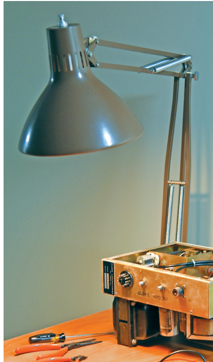
Figure 9 — This flexible light fixture can accept most common base bulbs, not just the incandescent ones it was originally designed for. A modern LED spotlight is a good choice.
