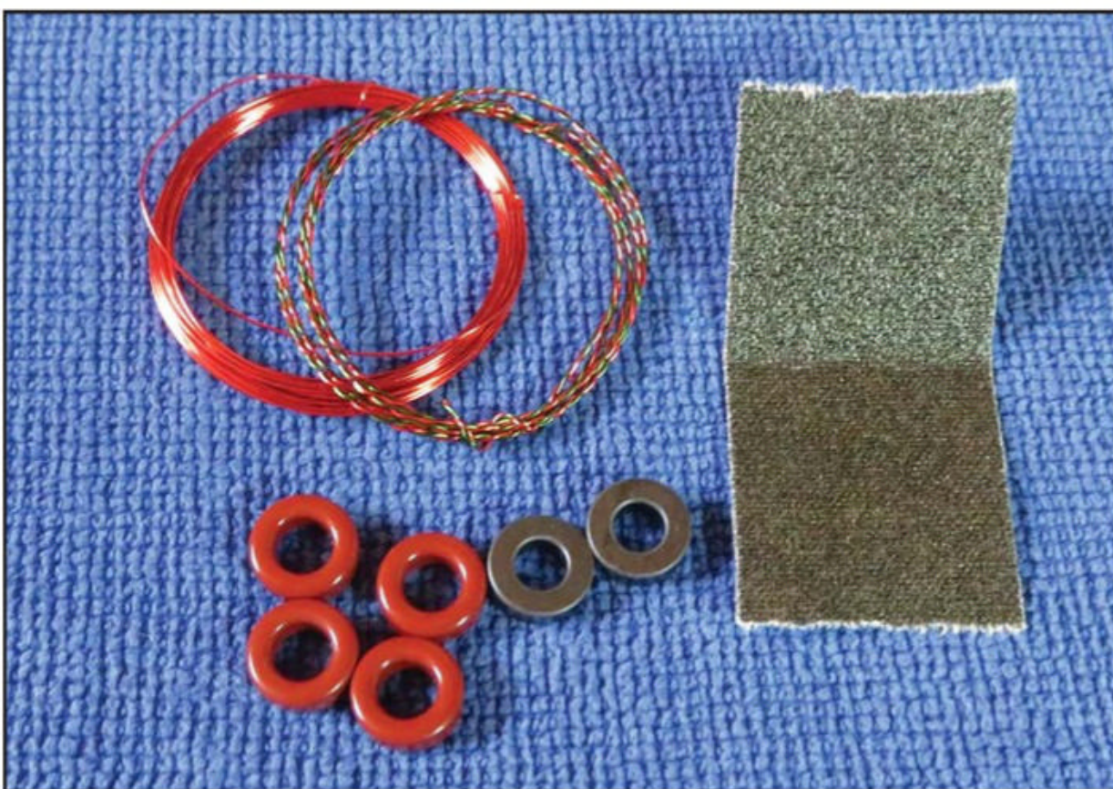
The six toroid cores and wire along with the supplied sandpaper ready to wind and prepare for mounting.
