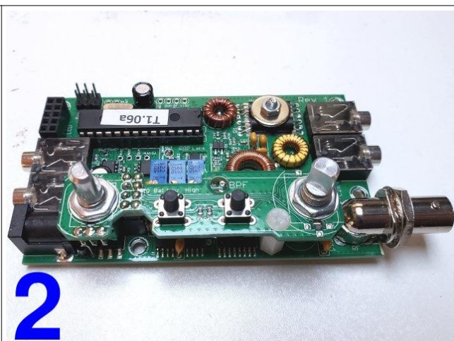
2 ... and the main board, with the controls board bolted in position.
