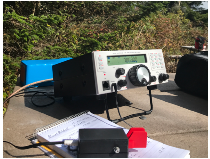
Mission RGO One Mt Mitchell State Park POTA: With a 15 aH LiFePo battery, you can operate CW for hours on end in the field.
