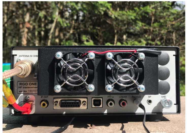
Mission RGO Back Panel: On the back panel you'll find standard Powerpole connectors for DC in, IF Out for pan adapters, ACC1 port, USB port, PTT in, Linear, Paddle, Speaker, and ports for future additions.
