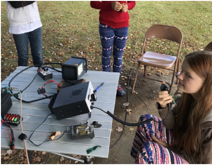
Mission RGO One Class 1 and Class 2: The Mission RGI One was the perfect HF radio to demonstrate 20-meter SSB DXing!
