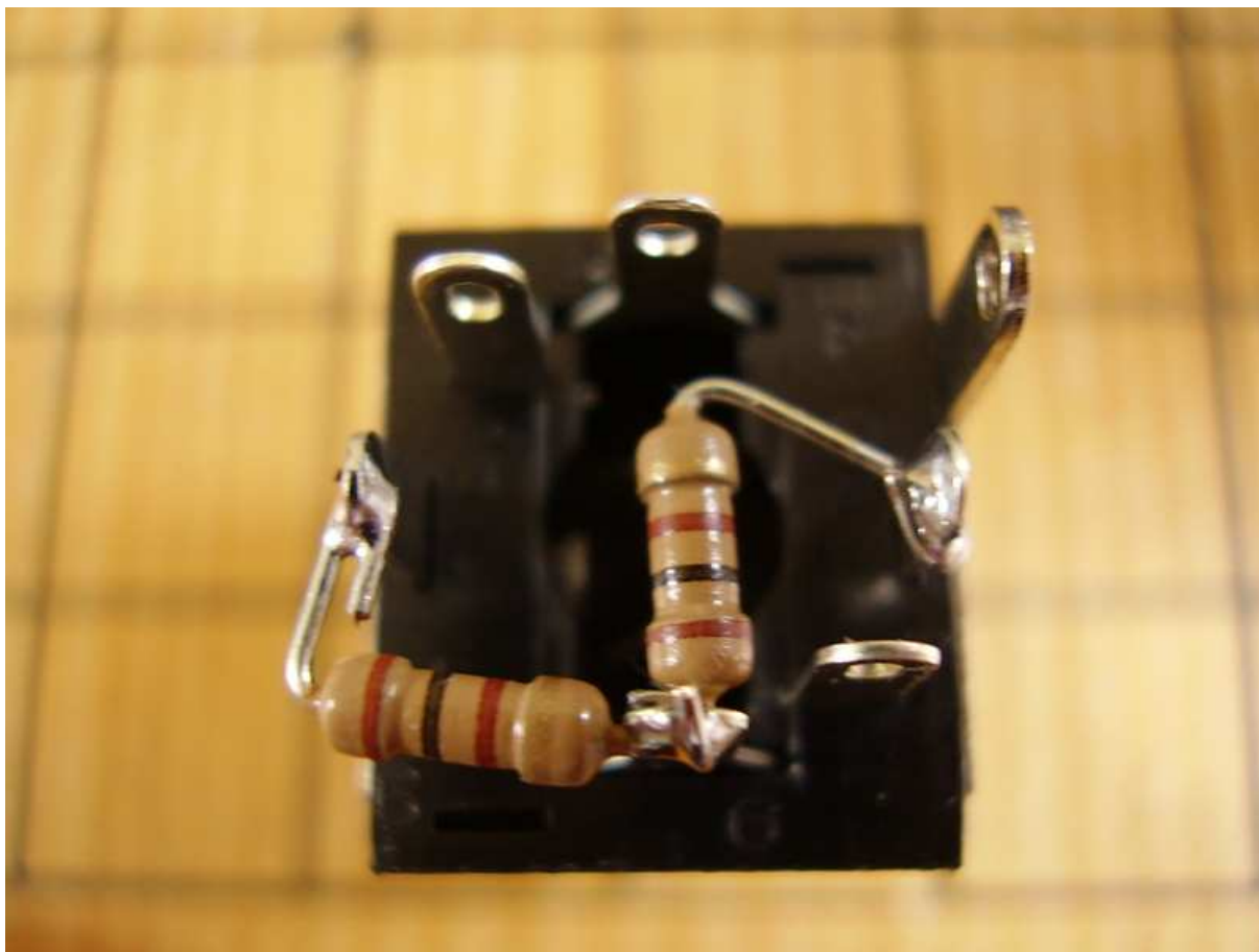
Figure 10.4: 100 Ohm Resistors Installed.
