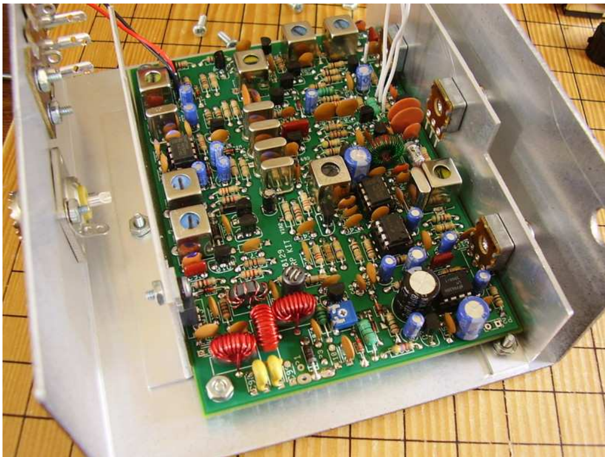
Figure 10.2: Board Installed in Center Shell.
