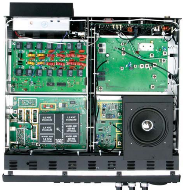
PHOTO 2. UNDERNEATH THE TOP COVER SHOWING IF, LPF AND SUB RX BOARDS
