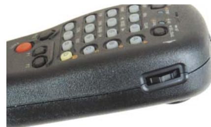
Figure 6— Tuning wheel on the side of the MH-59 Remote Control Microphone.
